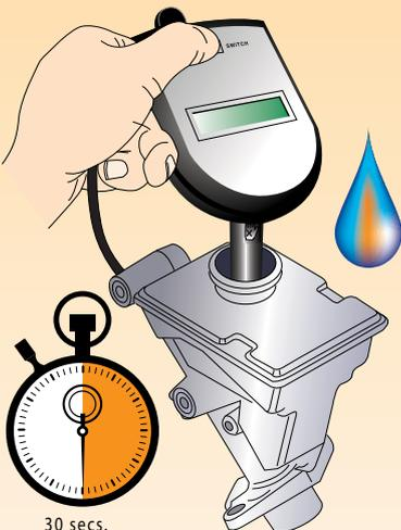
**FACT:** It only takes a minute... It takes less than a minute to check the boiling point of the brake fluid and identify those vehicles whose brake fluid has absorbed too much moisture to be safe.
